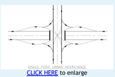
of traffic where streams of traffic merge or separate. The SPUI is a type of interchange where the arterial and ramp entrances/exits are controlled by a single traffic signal.
